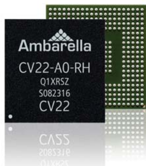
The CV22 chip targets sports, VR/360°, drone, and wearable camera designs
